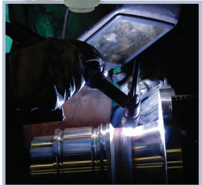
Welding a weld neck flange to a swivel joint sleeve in Chestertown, MD
